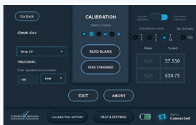
Select channel, cuvette and extraction ratio.
