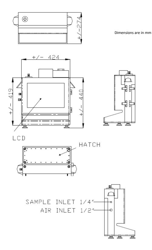
Process Imaging MEx1A General Arrangement Drawing
