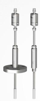
The Model 755<sup>™</sup> is an adjustable length, membrane tip probe regulator designed to sample transmission quality natural gas. The pressure regulator is built into the probe immediately downstream of the membrane, inside of the pipeline. Heat is transferred from the flowing pipeline gas to the regulator to prevent excessive JouleThomson cooling, helping to prevent condensation during pressure let down.
